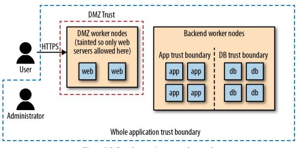
Figure 6-5. Sample container network controls
