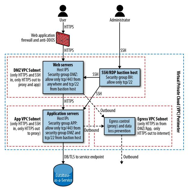
Figure 6-3. Sample application with network controls
