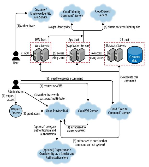
*Figure 4-3. Sample application diagram with IAM*
