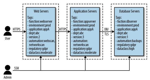
Figure 3-2. Sample application diagram with tags
